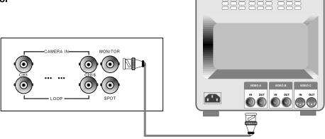
Connect the video output marked MONITOR to Video-In of Main monitor.
